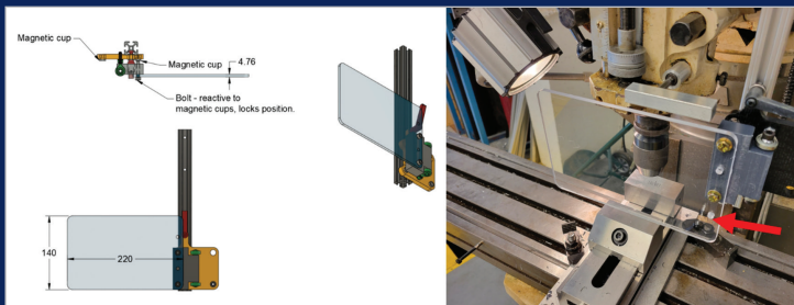
Physics Mechanical Technician Eric Fernandez designed and fabricated a custom guard for their milling machine
